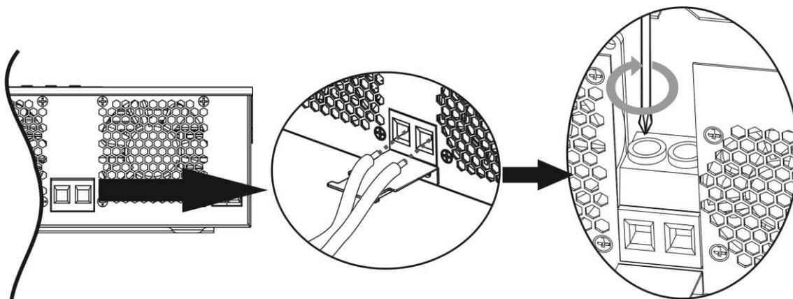
6. To firmly secure wire connection, you may fix the wires to strain relief with cable tie.
