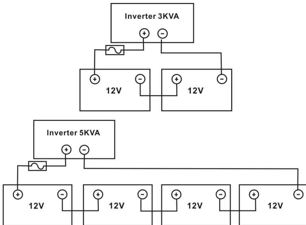
5. Insert the battery wires flatly into battery connectors of inverter and make sure the bolts are tightened with torque of 2 Nm in clockwise direction. Make sure polarity at both the battery and the inverter/charge is correctly connected and conductors are tightly screwed into the battery terminals.
