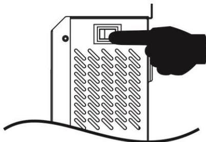
Once the unit has been properly installed and the batteries are connected well, simply press On/Off switch (located on the button of the case) to turn on the unit.
